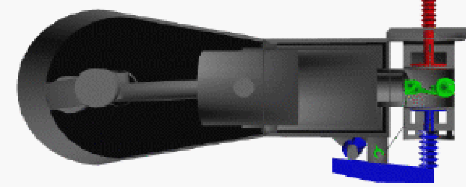
Stage 2 – Begin Compression Stroke
